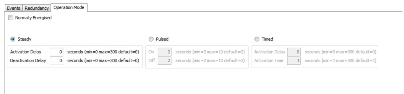
Instant: follows the status of the event: Active event: (detector in alarm) activated output (after any delay); event reset: output deactivated (after a period of delay).
