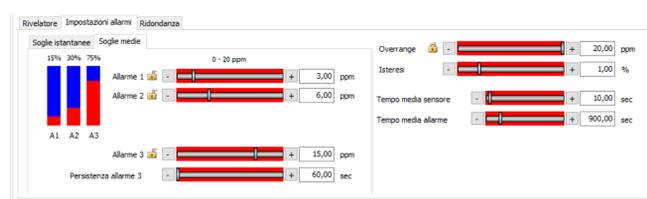
Alarm threshold settings and operating modes vary according to the selected Profile and Gas Type. There are two threshold modes, Average and Real-time.
